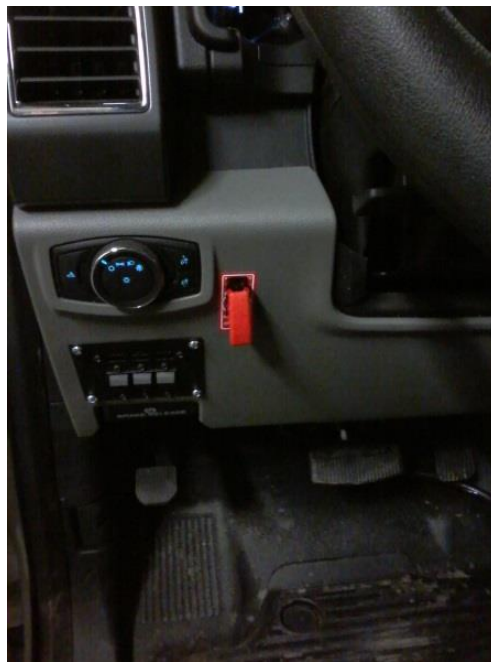
FIGURE 16: Top – Decal can be installed in two different orientations Bottom - Switch is installed on the dashboard
