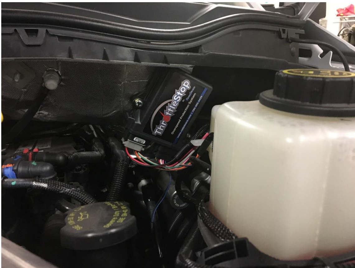
FIGURE 14: Installation of Throttlestop module on Ford 2017 6.7L
