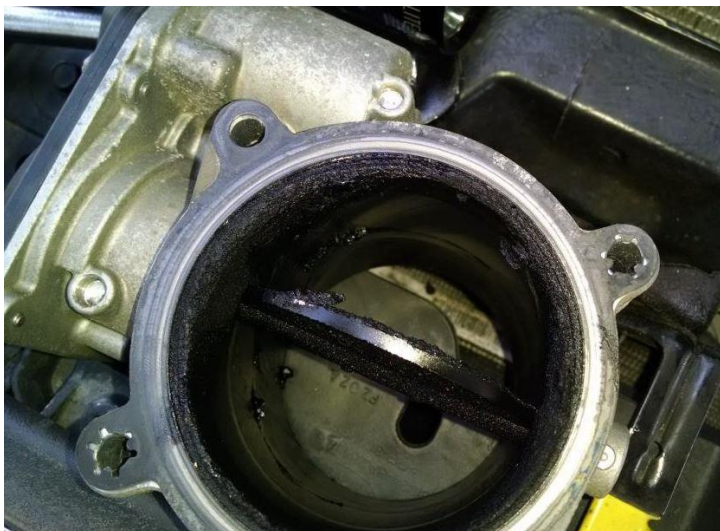
Figure B: Throttle valve with carbon build-up.
