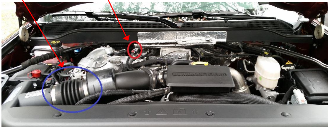
FIGURE 3: Location of valve port and crankshaft speed sensor on GM Engine
